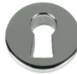
Round escutcheon 319 s/s 304 handpolished Diameter: 15 mm Thickness: 4,0 mm
